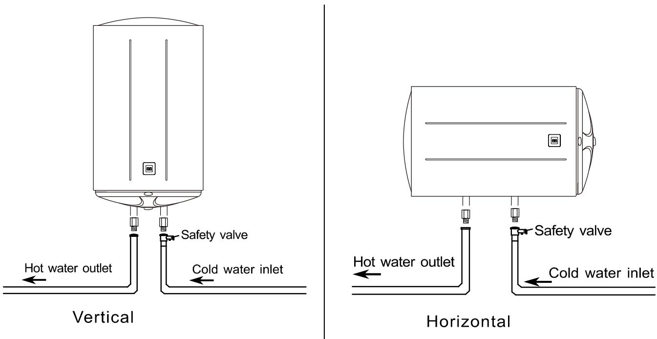
Thread the cold-water intake pipe (blue) to the electrolytic hose and from this to the hydraulic safety sub-assembly with the draining device supplied with the heater. Fit a cut-off valve to the cold-water supply pipe. **IMPORTANT: the cut-off valve must always be in the open position whenever the heater is switched on,**
