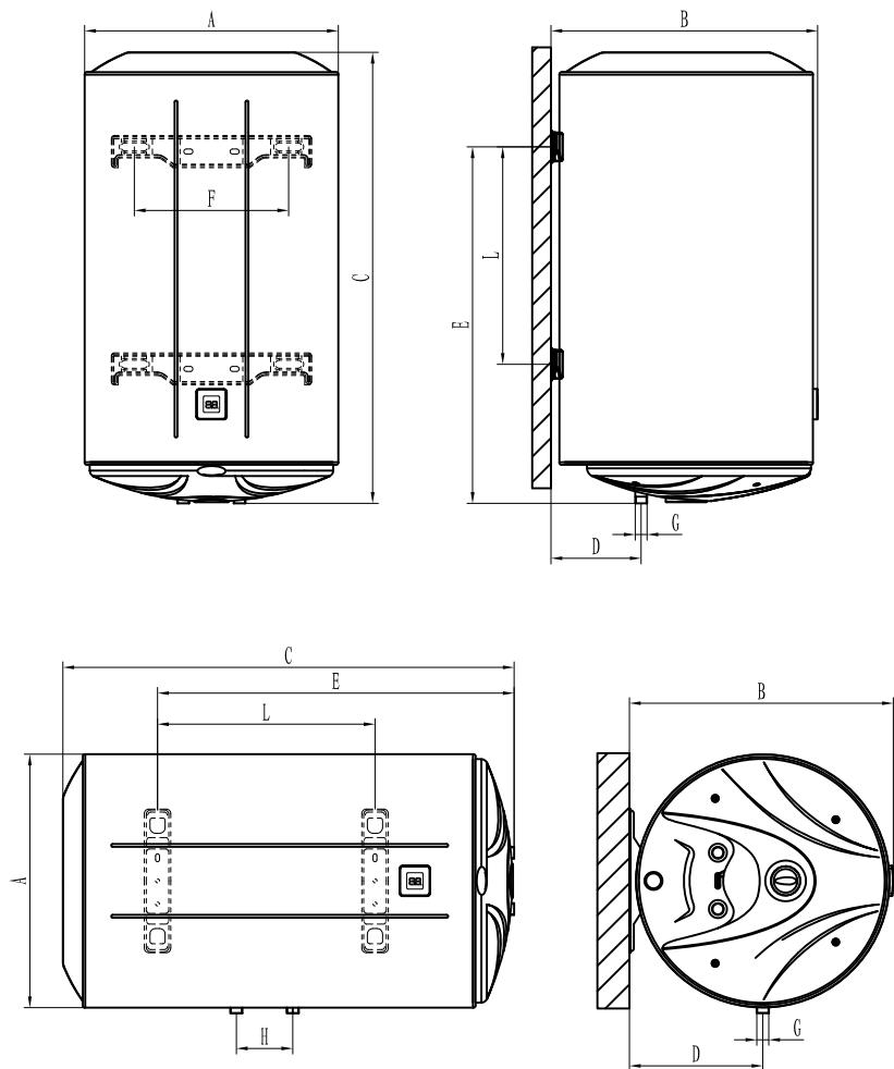
\*The TBL plus100-150L model has 2 metal mounting brackets.
