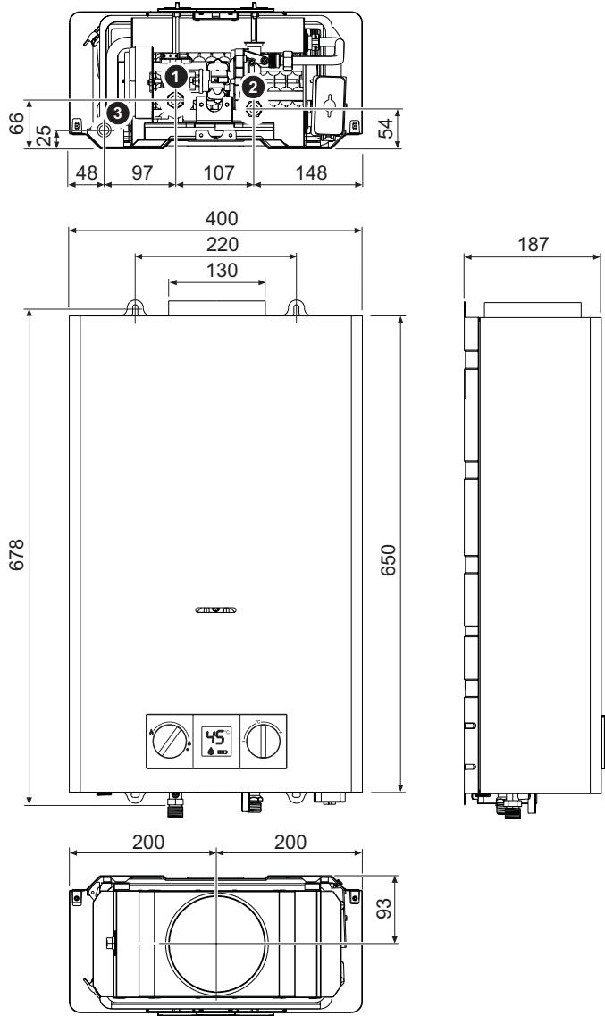
fig. 21 - Dimensions and connections CADI 14
