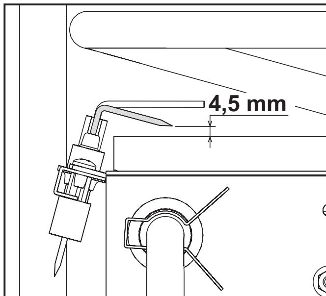
fig. 16 - Electrode position
