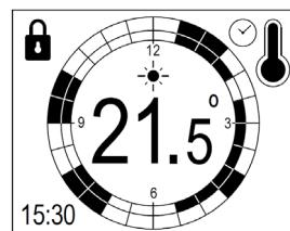
The program is displayed using a circle, which represents an analogue clock face. The screen automatically switches the display between the current time and the day of the week every 5 seconds.
