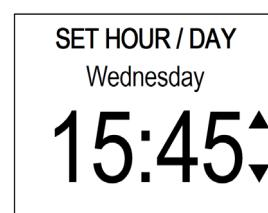
When the button cell battery life ends (see page 50), after a power failure or disconnection from the mains of more than one minute the emitter will request the user to set the hour/day, as the system clock is reset to Monday 00:00.
