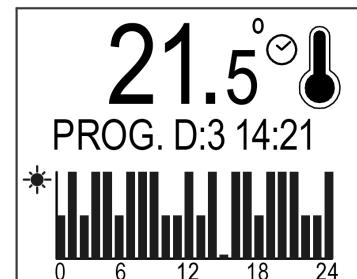
This function only runs when the emitter is in Program mode. When Adaptive Start is running a flashing clock icon is displayed next to the thermometer symbol. The mode will only function on temperature rise e.g., from heating off to eco / comfort, or from eco to comfort.
